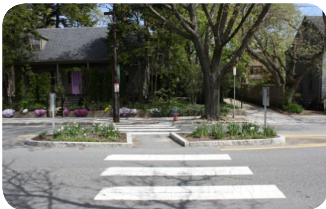
Figure 11. Examples of median refuge (left) and curb extension (right) to shorten crossing distances.
